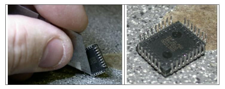
**Step 3**, Bend out pin-24 on the replacement prom like the picture below.
