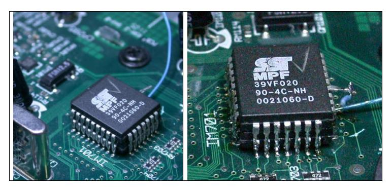
**Step 6**, Attach the longer wire to pin 32 of the stacked PROMS and the short wire to the eye-lit of the cut-trace.
