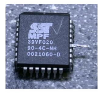
Step 4, Cut this trace connecting pin-24 on the main board and solder a short wire (1") to the old prom
