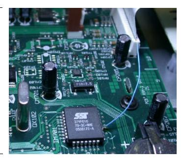
Step 5, Place the new modified PROM on top of the old one and check for good alignment of the leads, it should fit on top a little snug, if it is loose and moves around easily bend the leads further inward so you get a good snug fit. Then Solder all the leads (Except for pin 24) to the old prom. Should you create any solder shorts solder wick will easily fix you up. Solder a short piece of wire (1/2") to the pin-24 sticking out on the new PROM.
